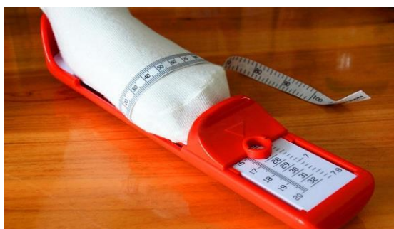
Fig. 2: Instrument for measuring the size and perimeter of the fingers of the human foot
